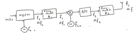
The desired (target) carrier frequency  $f_c$  is 100 MHz and frequency deviation  $\Delta f = 75$  kHz the message signal to be broadcast is given by:
